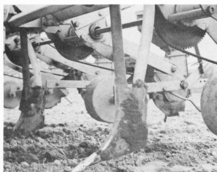
Figure 5. Chisel point furrow opener for placing fertilizer.
