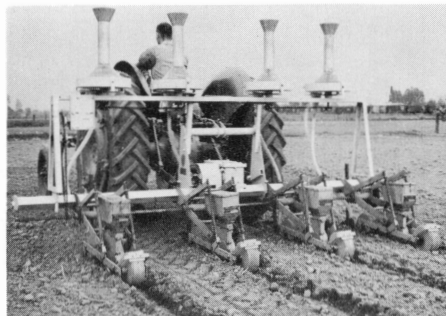
Figure 2. Plot seeder and fertilizer applicator mounted on a three-point hitch.
