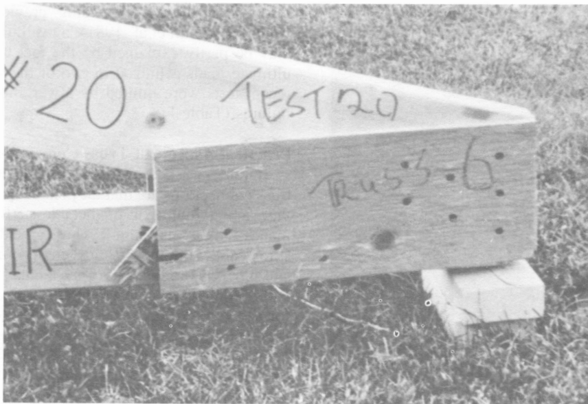
Figure 5. Another series C four-ply D. fir plywood failure, due to rolling shear delamination within the two vertical center plies.
