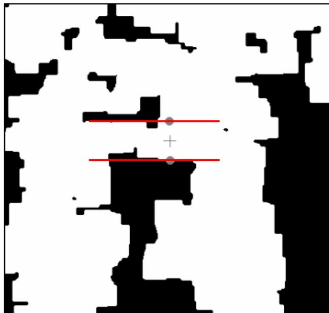
Fig. 7. Example of error in determination of stripe location by the Stripe Analysis algorithm in a field image: + = stripe centre; • = stripe edges.
