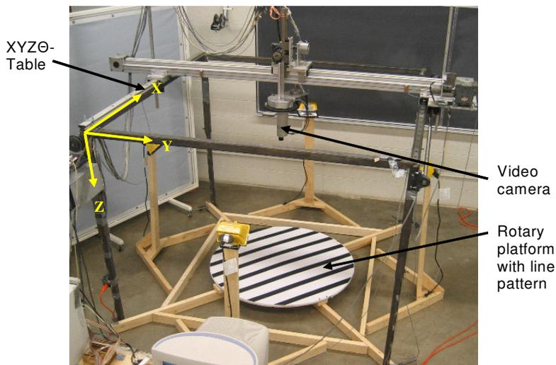
**Fig. 2. Line-detection algorithm testing set.**
