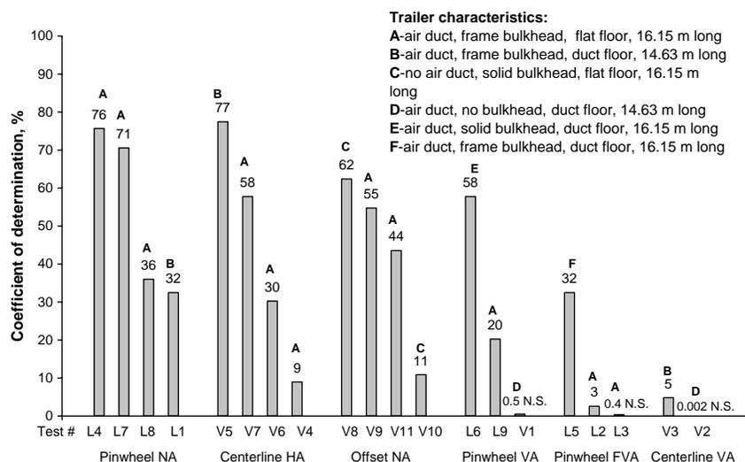
**Fig. 4. Air distribution in semi-trailers, grouped according to loading pattern and use of air bags ( $p = 0.10$ ).**
