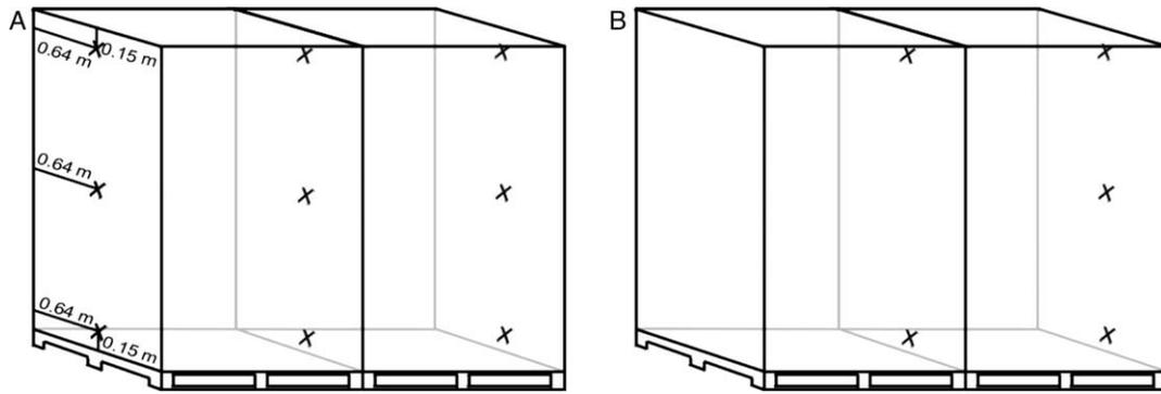
Fig. 2. Location of data loggers on produce pallets in the first 3 tests (2A) and the remaining 17 tests (2B).
