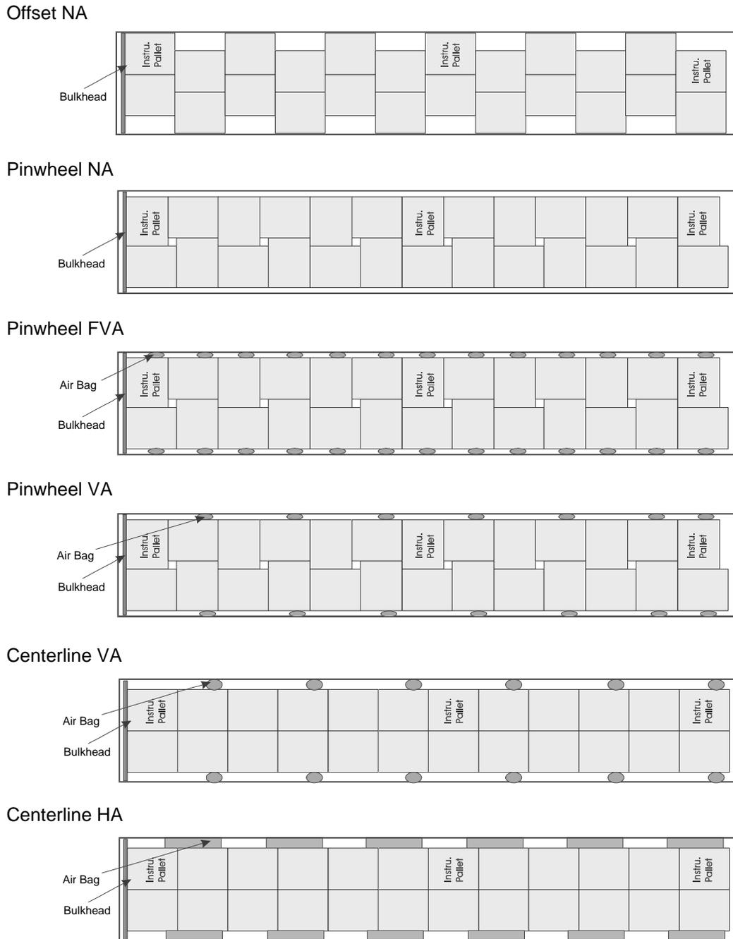
**Fig. 1. The loading and bracing patterns used in the field tests. The actual locations of the instrumented pallets may vary depending on the number of produce pallets in the load and the length of the trailer.**
