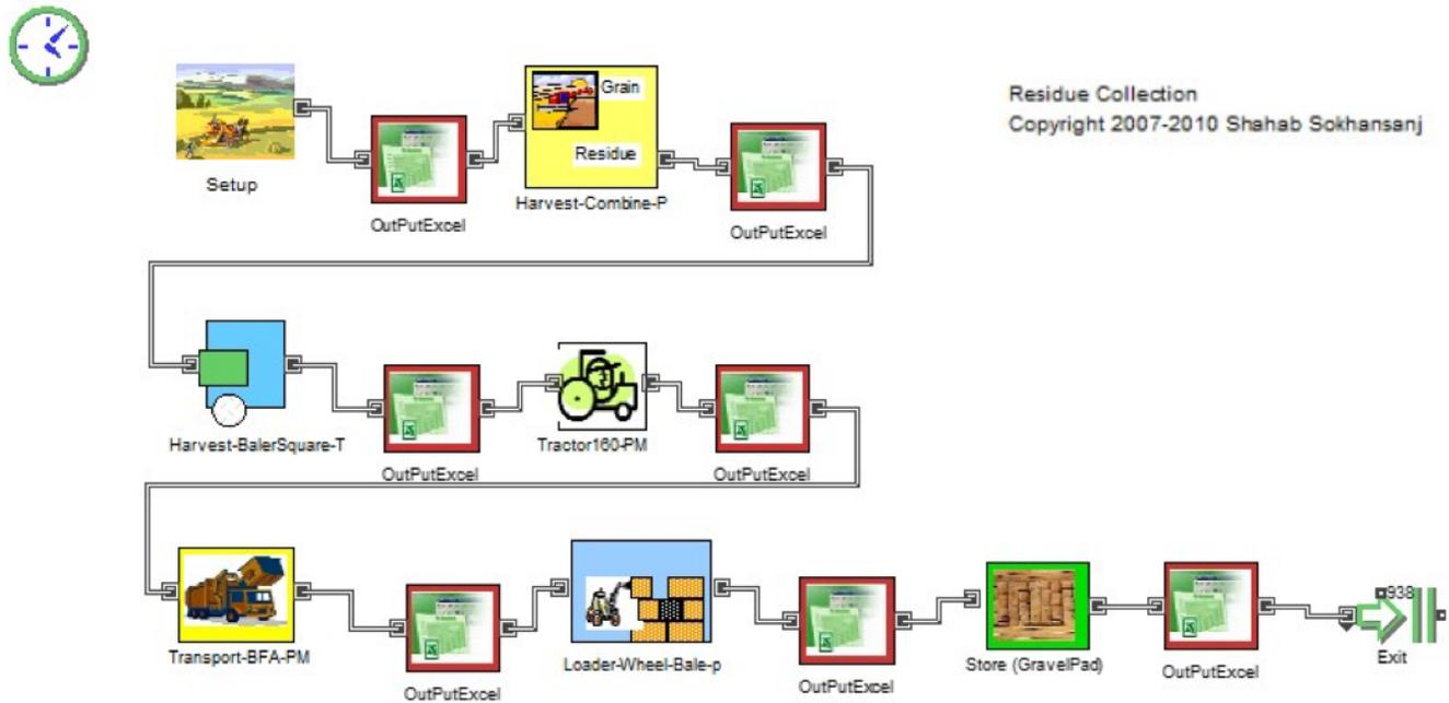
**Fig. 2. Image of IBSAL modules assembled for wheat straw harvest. The system consists of combining, baling, transporting bales to the side of the farm and stacking bales on prepared graveled ground. The bales are tarped to prevent from rain damage.**
