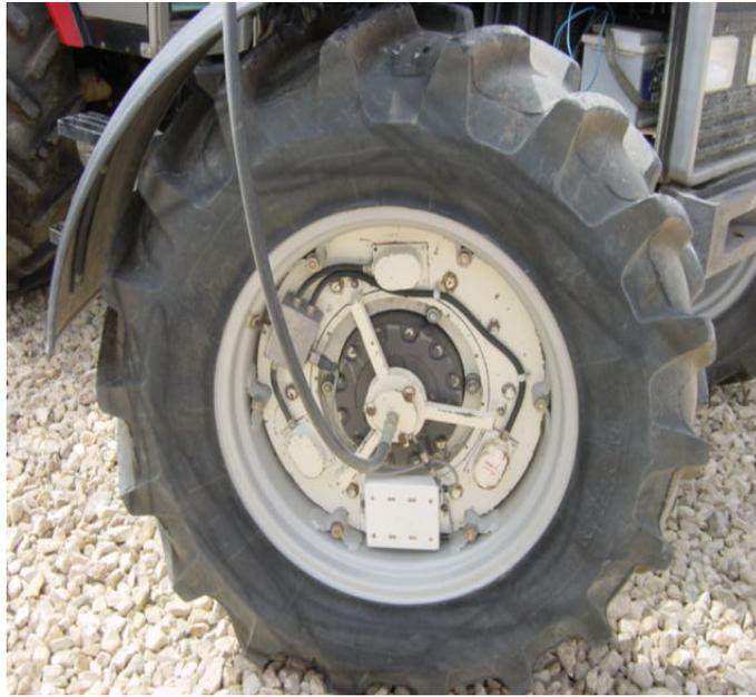
Figure 2. Tractor wheel fitted with the wheel torque and weight transducer.
