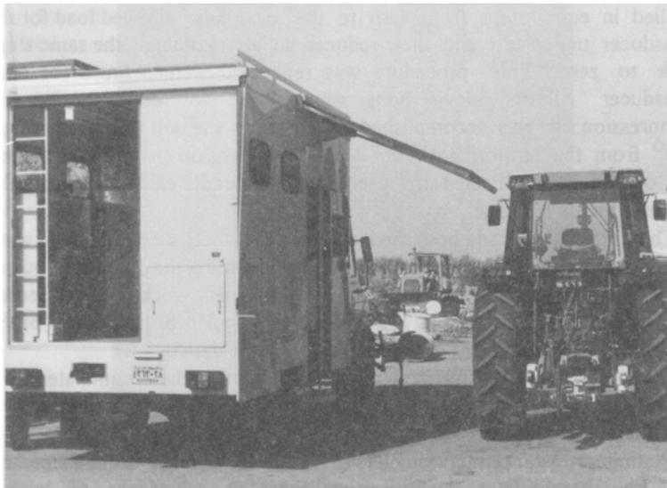
Figure 3. Overall view of the mobile instrumentation lab and the MF-3090 instrumented tractor.
