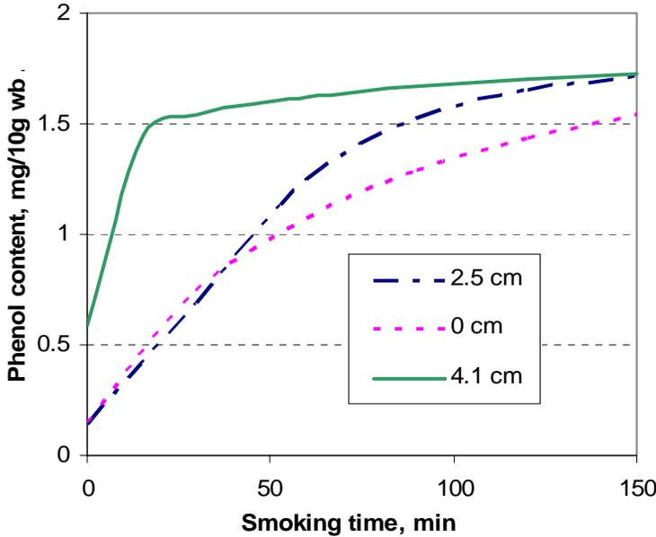
Fig. 6. Simulation results of the phenol distribution across a 9 cm block of cheese. The dotted, dashed-dot, and solid lines show the phenol content change during smoking in a layers located 0, 2.5, and 4.1 cm from the centre of the 9 cm thick block of cheese. The simulation was conducted for the effective diffusivity of  $0.1 \text{ cm}^2/\text{min}$ .
