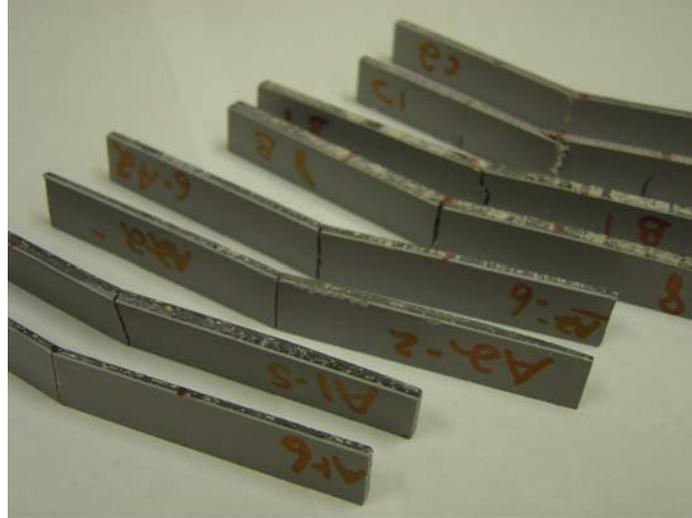
Figure 5. Failure pattern of flexural strength specimens after test
