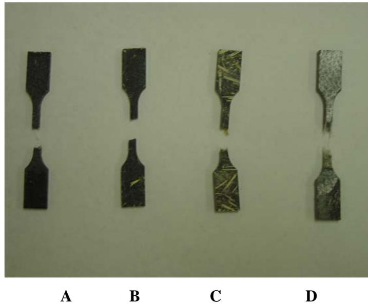
Figure 4. Failure pattern of tensile impact strength specimens after test
