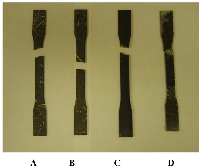
Figure 3. Failure pattern of tensile strength specimens after test
