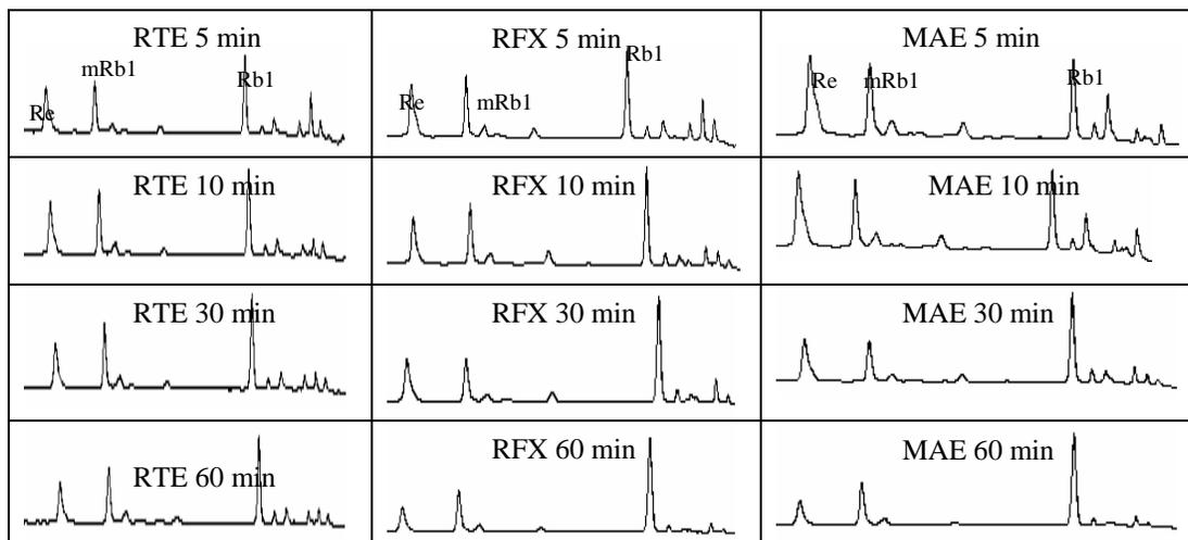
Figure 9: Chromatographs of ginseng root extracts obtained using different extraction methods and extraction times
