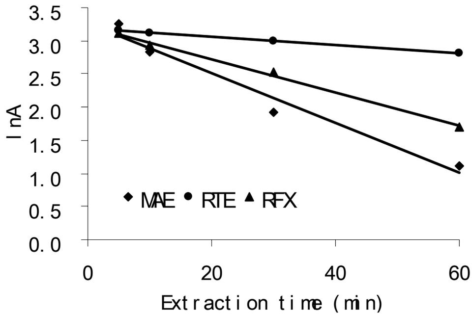
Figure 7: Linear regression of lnA vs. extraction time for ginsenoside Rb1 using the three extraction methods.
