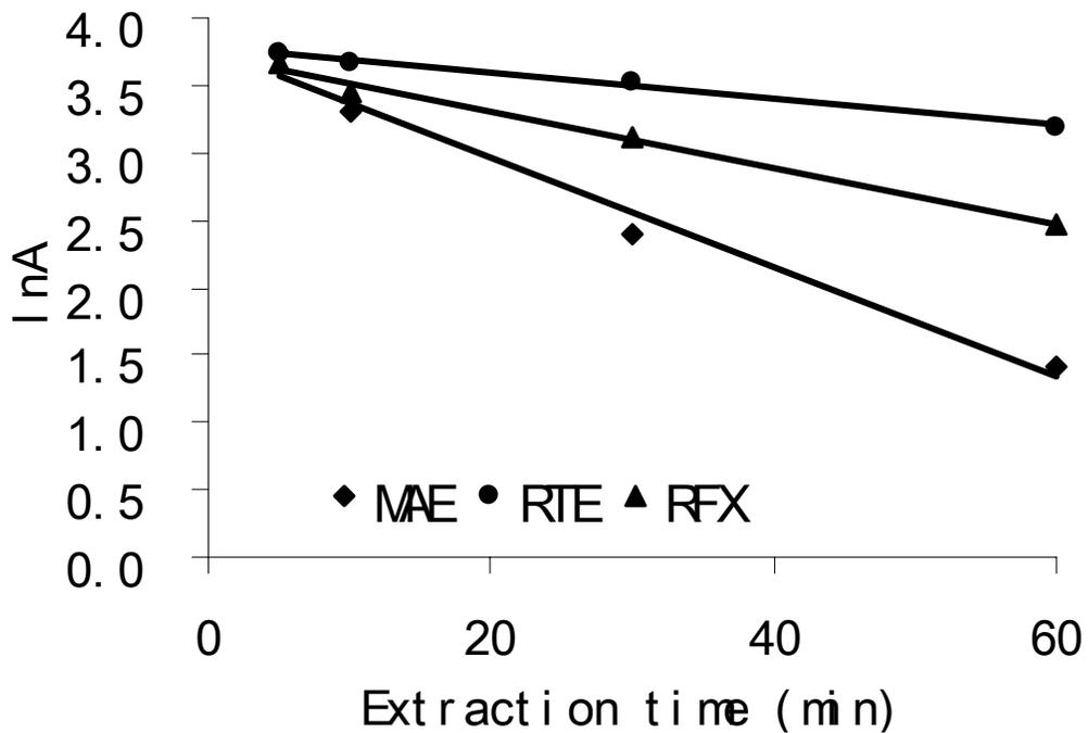
Figure 8: Linear regression of lnA vs. extraction time for total ginsenosides using the three extraction methods.
