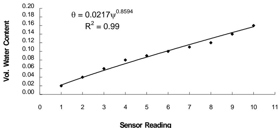
Figure 2. Chart of Sensor Calibration
