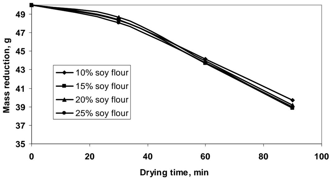
Figure 3. Microwave drying of mango fruit leather at 6 power level (12 W/g)
