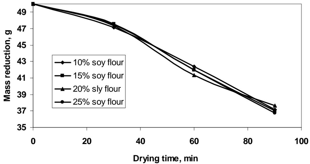
Figure 4. Microwave drying of mango fruit leather at 8 power level (16 W/g)
