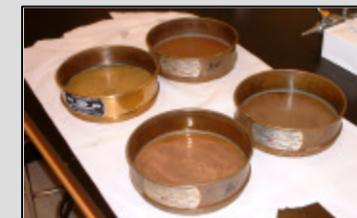
Fig. 4 – Soil screens used to find particle size distribution – mesh sizes were: 18, 60, 100 and 350 (i.e. openings per 25.4 mm)
