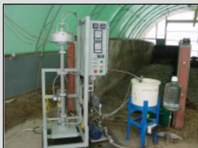
Fig.1 – VSEP test unit equipped with reverse osmosis filter pack.
