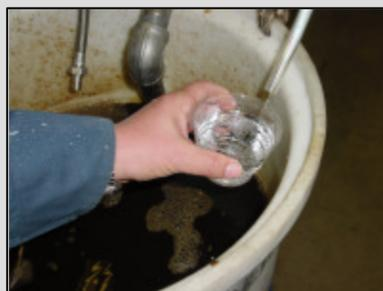
Fig. 2 – Recovery of water from VSEP unit (liquid manure input)
