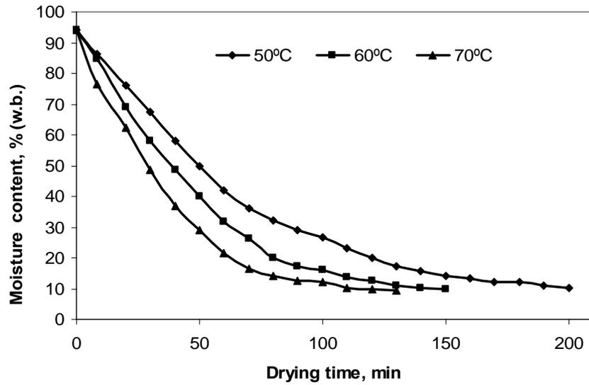
**Figure 6. Relationship between moisture content and drying time of microwave assisted hot air drying of tomato slices**
