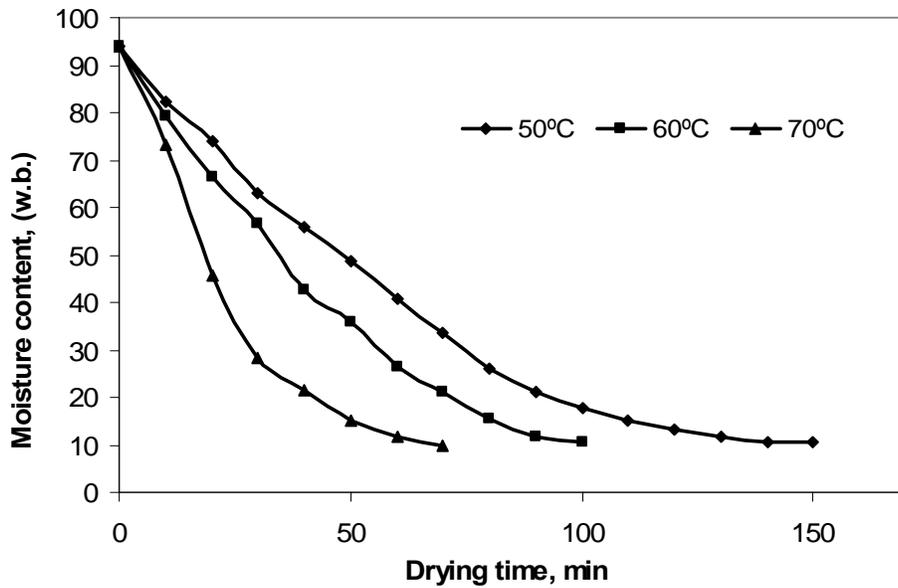
**Figure 4. Relationship between moisture content and drying time of microwave assisted vacuum drying of tomato slices**
