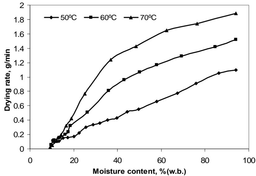
**Figure 7. Relationship between drying rate and moisture content of microwave assisted hot air drying of tomato slices**
