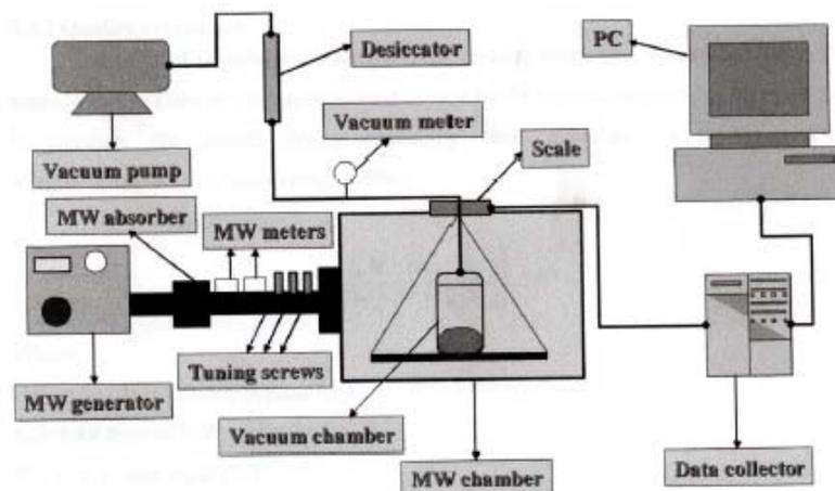
**Figure 1. Schematic view of microwave drier set up**
