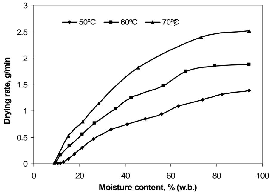
**Figure 5. Relationship between drying rate and moisture content of microwave assisted vacuum drying of tomato slices**
