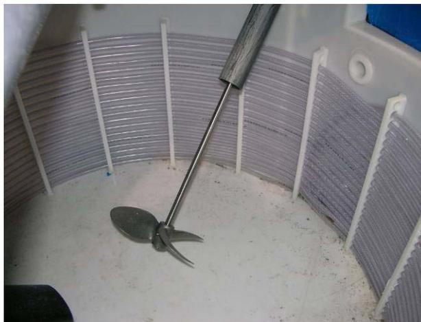
**Figure 3 Mixer installed in digester**
