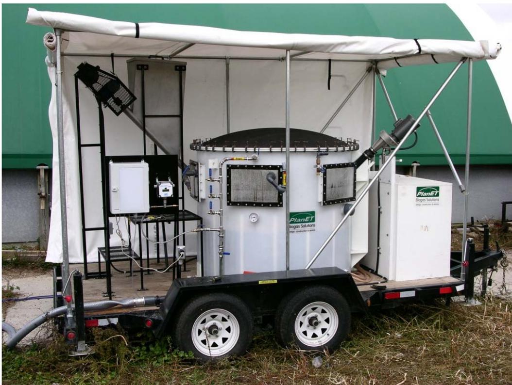
**Figure 1 Completed anaerobic digester**
