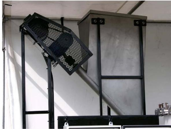
**Figure 4 Inclined auger and stainless steel hopper**
