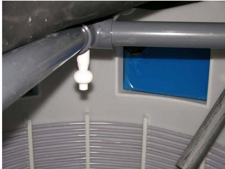
**Figure 8 Internal rinsing system to keep viewing windows clean**
