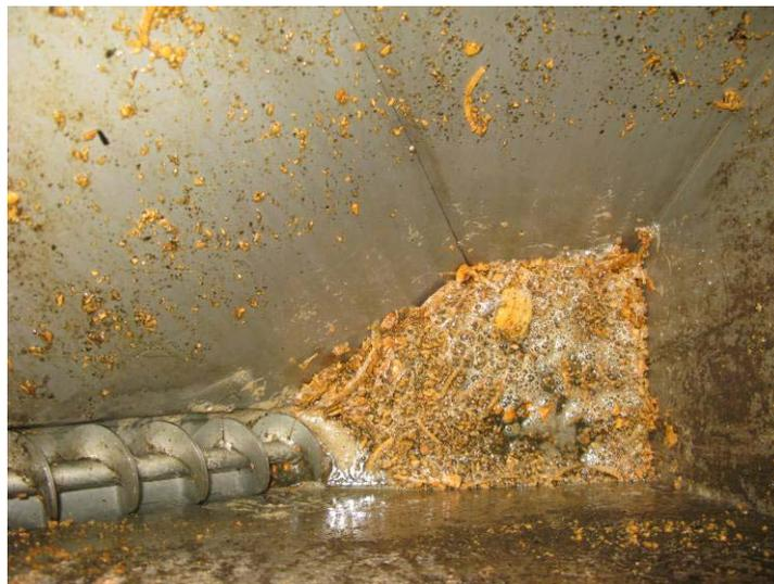
**Figure 5 Shredded sweet potatoes and recycled digestate being added through the auger**
