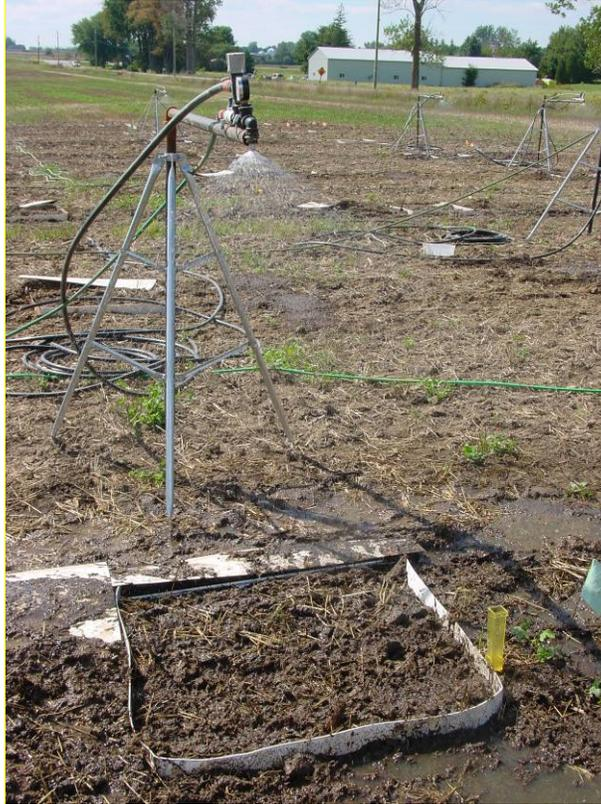
**Figure 3 Typical rainfall simulator test setup**
