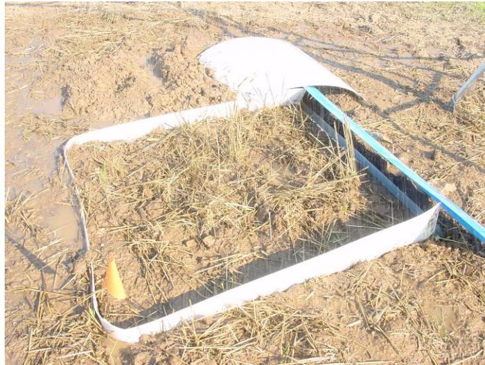
**Figure 1 Plot configuration in 2007 study, showing boundaries and covers over the collection trough and tub**
