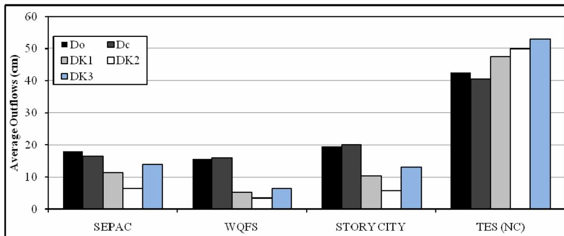
Figure 1. Observed and DRAINMOD-predicted yearly drainage volumes using  $K_{sat}$  values estimated by group 1 PTFs.
