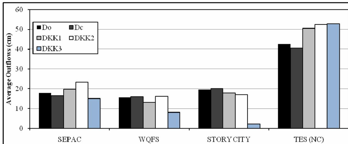
Figure 2. Observed and DRAINMOD-predicted yearly drainage volumes using  $K_{sat}$  values estimated by group 2 PTFs.
