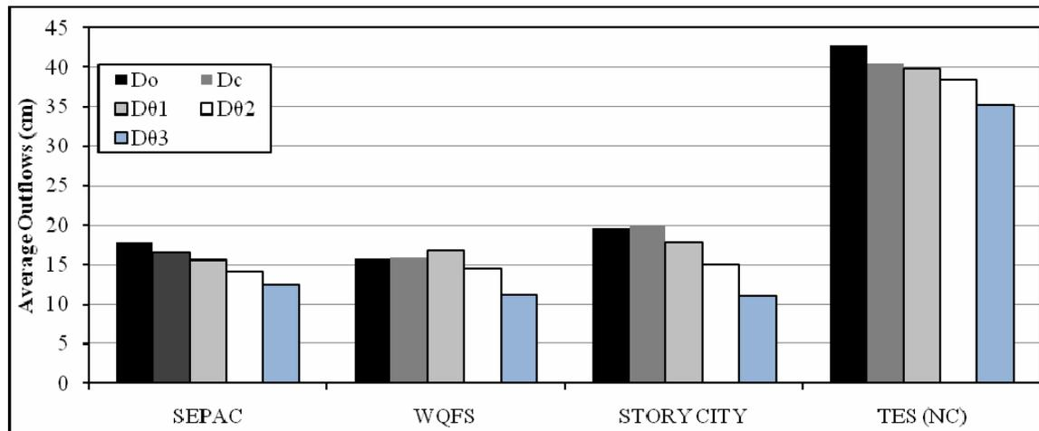
Figure 3. Observed and DRAINMOD-predicted yearly drainage volumes using SWC data estimated by PTFs.
