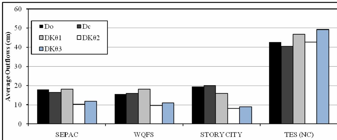
Figure 4. Observed and predicted outflows using  $K_{sat}$  and SWC data predicted by PTFs
