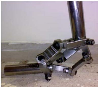
Fig. 4. A sample of proposed mechanism that can rotate to a crossover angle of 135 degrees.
