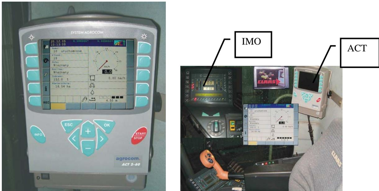
Figure 1. Control panel of an on-board computer for harvest registration in the Claas Lexion 480 combine.
