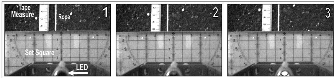
This uncertainty is reduced by using a high-speed camera (Pixelink™ PL-A741-E) on a mounting frame applied to a John Deere 6000 series tractor (Figure 4). The camera takes
