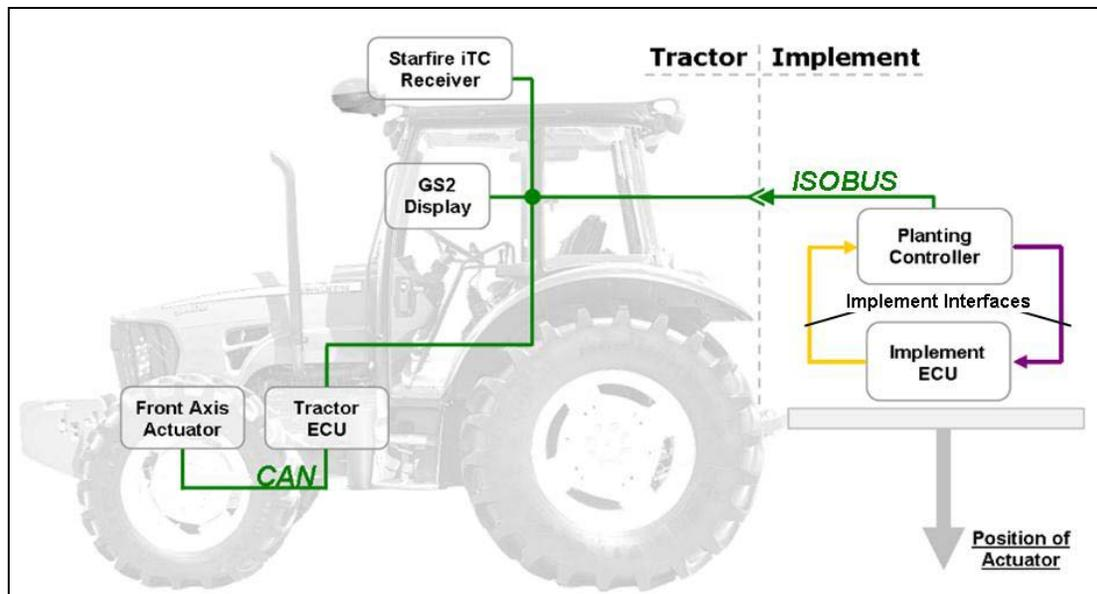
**User Interface** The Planting Controller has its own ISO 11783 compliant Virtual Implement (VI) and Task Controller. These features allow to configure all needed pattern parameters and the documentation of the triggered positions.
