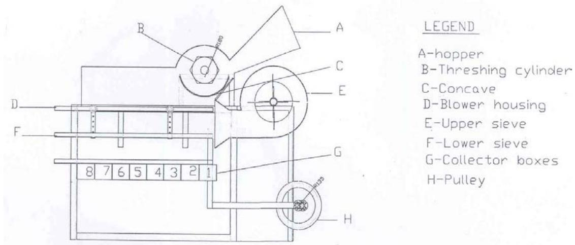
Figure 3. Sectional view of the sorghum thresher testing rig.
