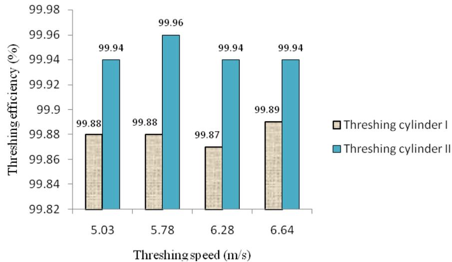
Figure 5. Threshing efficiency of the two threshing cylinders
