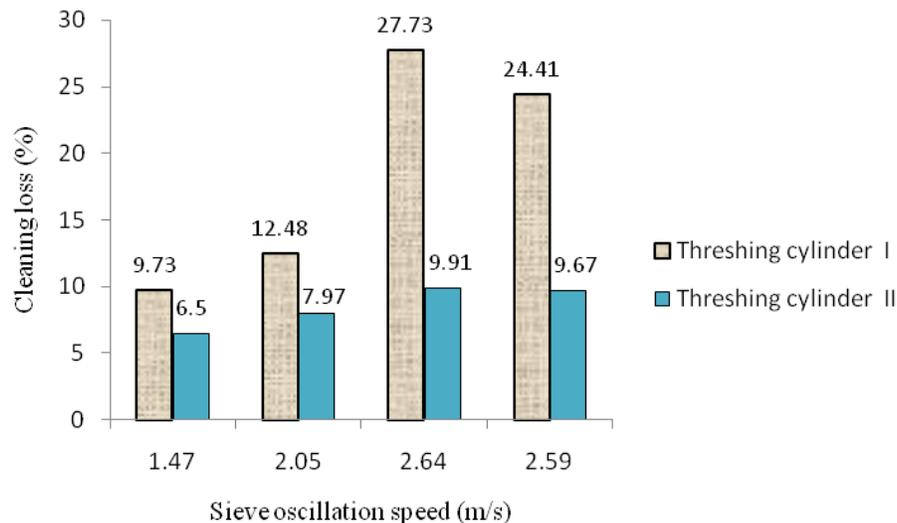
Figure 7 Cleaning loss from the threshing cylinders
