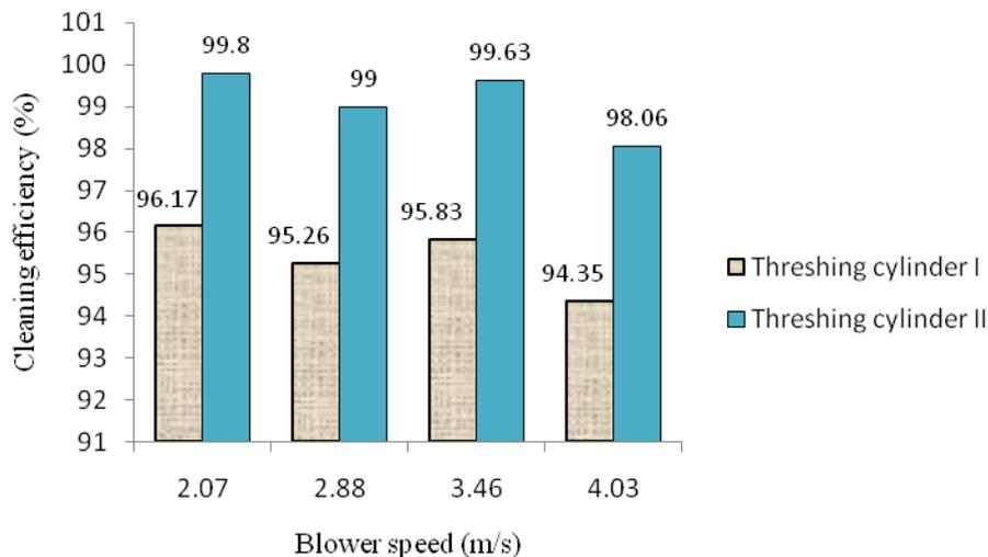
Figure 6. Cleaning efficiency of the two threshing cylinders
