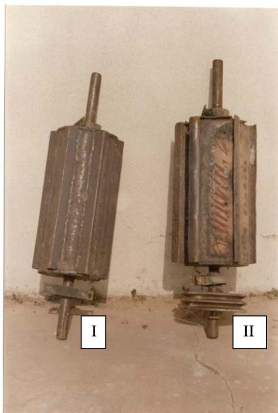
Figure 3. Threshing cylinders used on the sorghum test rig
