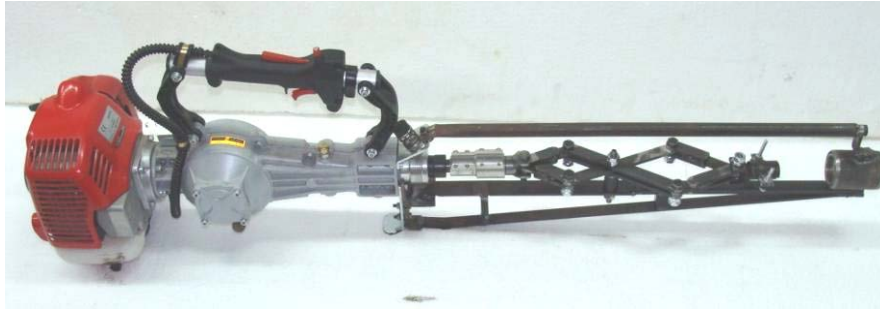
Figure 1. The hand-held shaker and the the amplitude changing mechanism used for shake harvesting trials. (shaker boom and hook not shown).
