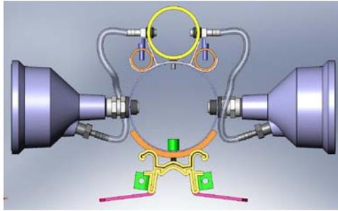
Figure 4 Cross-section of the foam generator assembly apparatus (ref: Sunarc of Canada)
