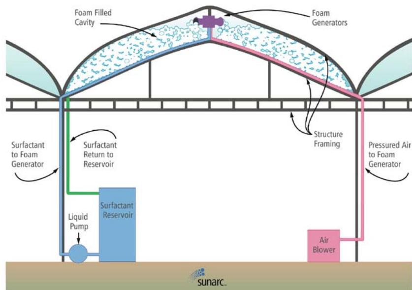
Figure 1 Cross-section view of multi-section greenhouse installation of a Sunarc System
