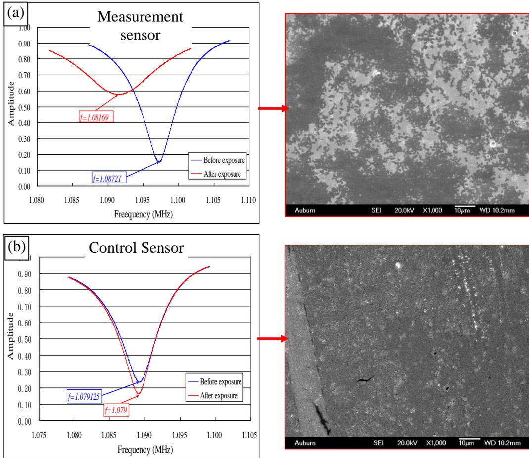
Figure 2. Typical resonance frequency shifts and the corresponding SEM images of the sensor surface for (a) the measurement ME biosensors and (b) the control sensor, as the sensors were placed on the spinach leaf spiked with *Salmonella typhimurium* suspension with the concentration of  $5 \times 10^8$  cfu/mL
