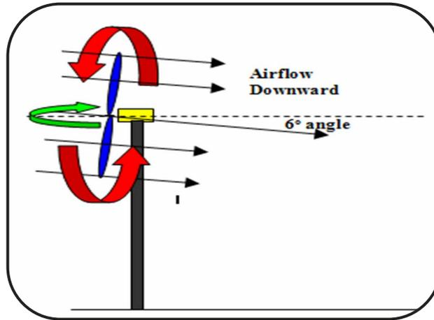
Figure 2. Wind machines pull warm air down from high above crop, blowing it downward and outward, pushing away cold air and replacing it with warmer air near target crops.
