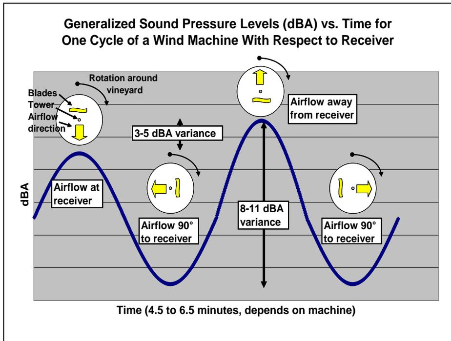
Figure 6. Neighbours hear wind machine sound as varying sinusoidally as blades sweep around the field. Sound is greatest when blades blow air *away* from neighbours, next greatest when blowing *at* them. If air is blown perpendicular, the sound is greatly reduced.
