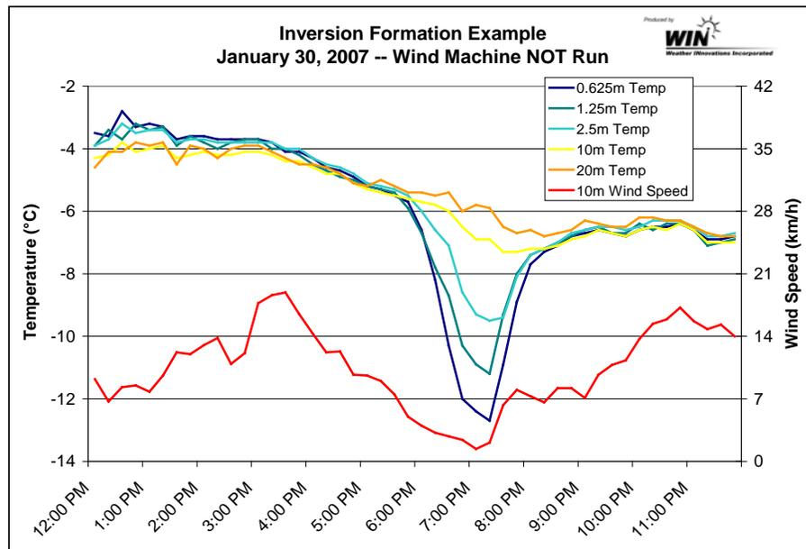
Figure 3. This strong temperature inversion below Escarpment near Virgil of about 7°C between 20 m above and 0.625 m above ground, started forming as winds dropped below 7 km/h at 5:30 pm. The inversion ended when wind speed rose above 7 km/h at 8:00 pm.
