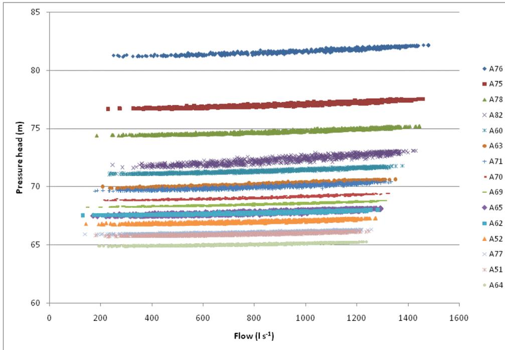
Figure 4. Effect of sequentially removing the critical hydrants on the pressure head requirements at the pump station
