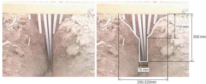
Figure 4. Rear view of soil disturbance for the sensor with the shank width of 18 mm and equipped with three sensing tips at depths of 100, 200 and 300 mm and operated at depth of 300 mm (WC=11.8%). Below the critical depth, the width of compacted zone is equal to the shank width. The direction of travel is perpendicular to plane.
