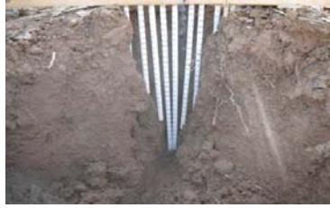
Figure 2. Soil disturbance pattern, the dimensions of the exposed profile was quantified using a profile meter.
