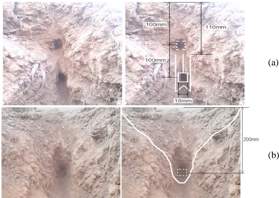
Figure 6. Photograph of developed channels with square cross-sectional area for the sensor a) with the shank width of 18 mm and with two sensing tips at depths of 100 and 200 mm, operating at depth of 200 mm (WC=12.7%) and b) with the shank width of 36 mm and with two sensing tips at depths of 100 and 200 mm, operated at depth of 200 mm (WC=10.8%). The squares with solid and broken lines edges are traces of prismatic tips in undisturbed and disturbed soil s, respectively. The direction of travel is perpendicular to plane.
