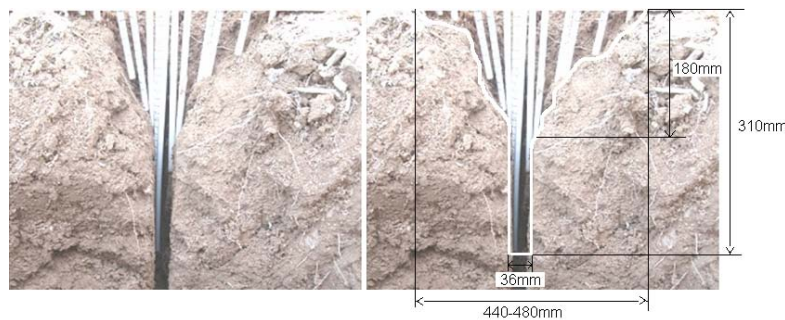
Figure 5. Rear view of soil disturbance for the sensor with the shank width of 36 mm and equipped with three sensing tips at depths of 100, 200 and 300 mm and operated at depth
