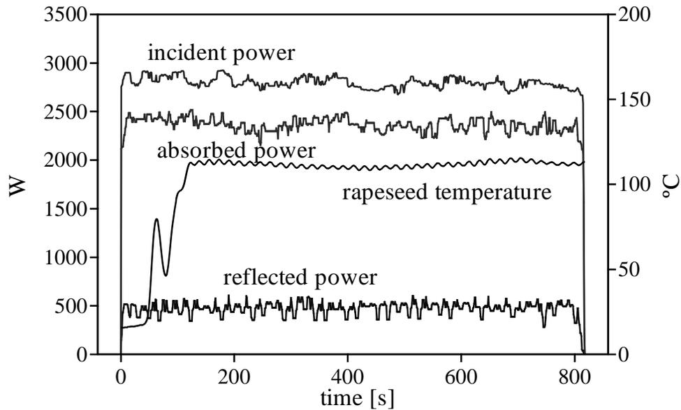
Figure. 3 Rapeseed temperature and incident, reflected and absorption power of microwaves
