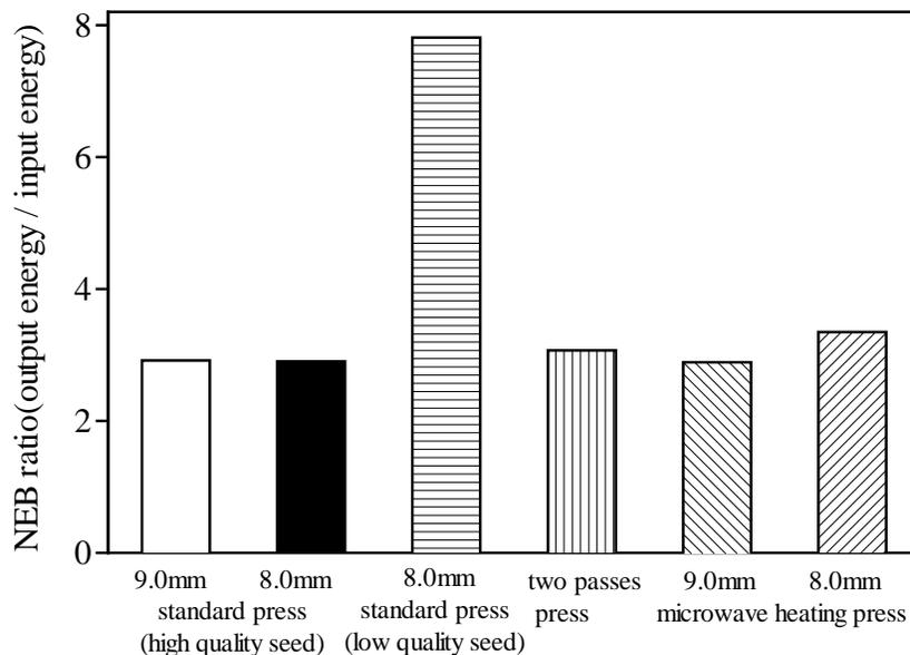
Figure 4. Net energy balance ration for biodiesel production
