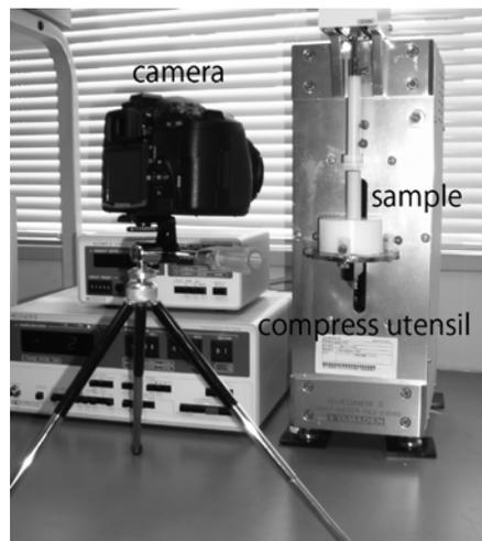
Figure 2. Photograph of measuring system.
