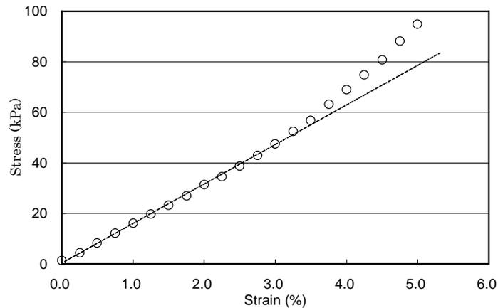
Figure 3. Stress-Strain curve for the cylindrical sample of fresh Japanese radish.
