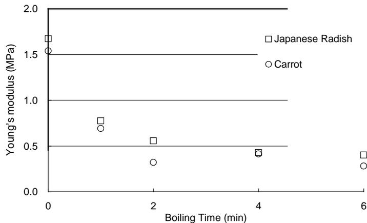
Figure 5. Changes in the Young's modulus for the cylindrical samples of Japanese radish and carrot during boiling.
