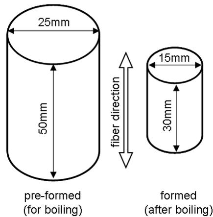
Figure 1. Schematic diagram of cylindrical samples.
