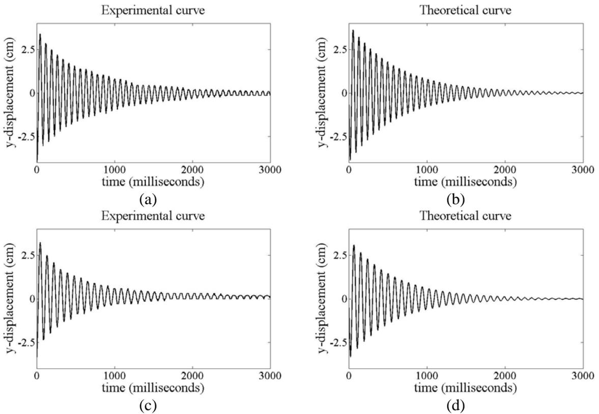
Figure 4. Decay oscillation curves for Catuai Vermelho variety (a and b) and for Mundo Novo Variety (c and d).
