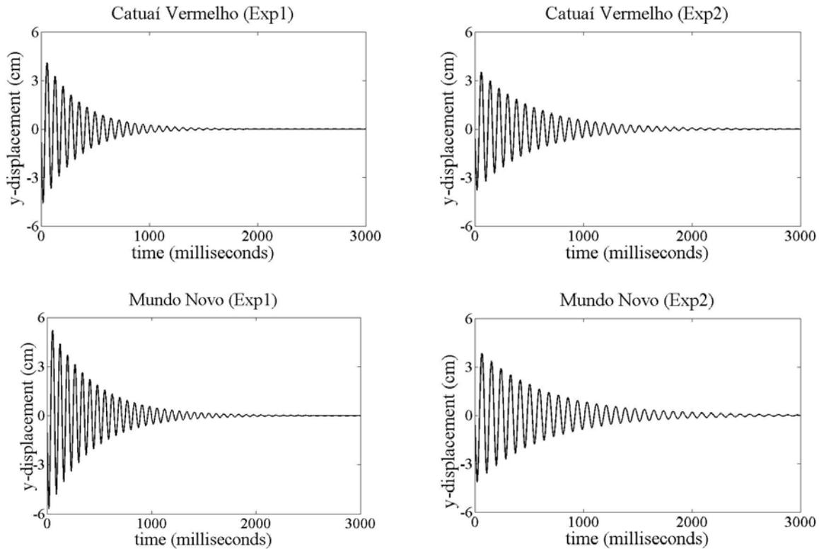
Figure 5. Decay curves for the average oscillation for both varieties and both experiments.
