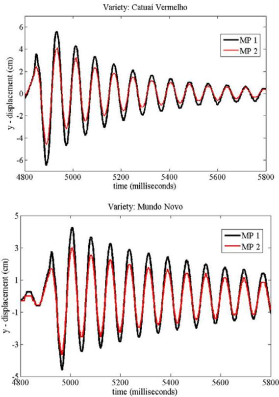
Figure 3. Decay curves for two different monitoring points for branches of both varieties.
