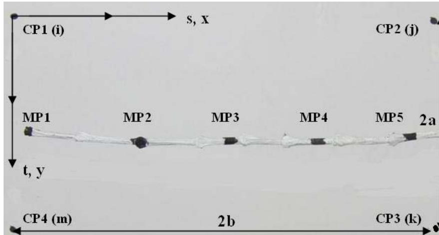
Figure 1. Coffee branch painted with monitoring points and background image with control points in test
