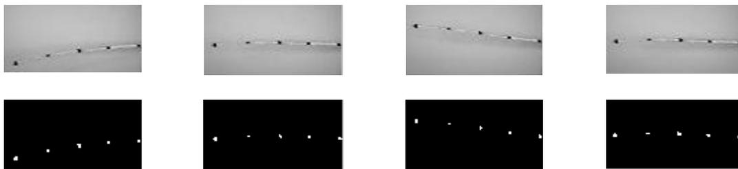
Figure 2. Gray scale images (upper part) and processed images (down part) showing the monitoring points in one of the performed tests
