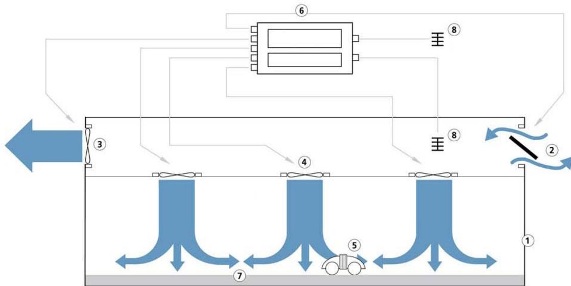
Figure 1 Scheme of the hybrid solar/waste-heat drying plant: 1) closed transparent hall, 2) ventilation flap, 3) exhaust fan, 4) ceiling fans 5) electric mole™ 6) PLC control system, 7) drying area, 8) sensors for temperature, relative humidity wind and global radiation (Starcevic 2003)
