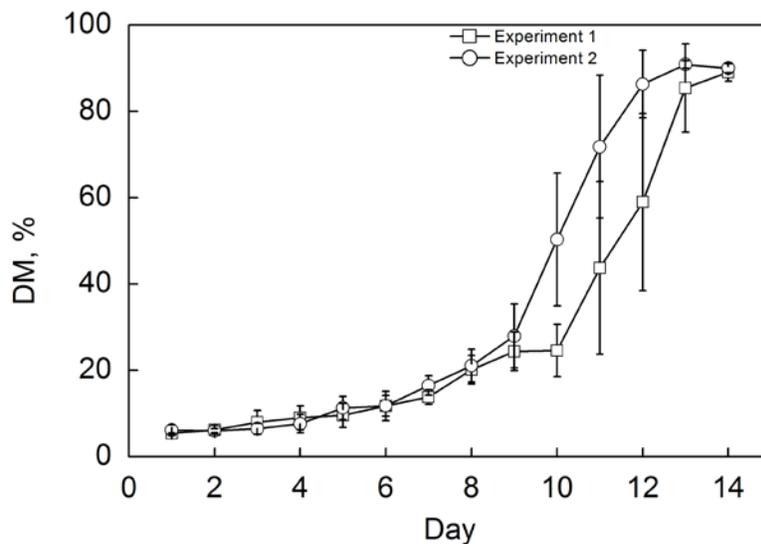
Figure 2 Changes in the dry matter content (DM) during drying (error bars indicate standard deviation).
