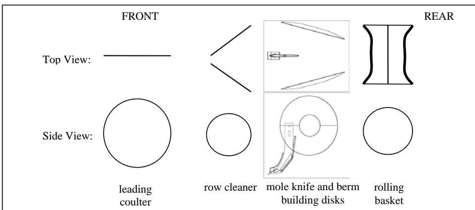
Figure 2. Top and side view schematic of a typical strip tillage row unit.
