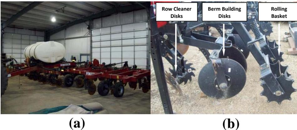
Figure 3. 'a' strip tillage equipment. 'b' side view of a single strip-tillage unit.
