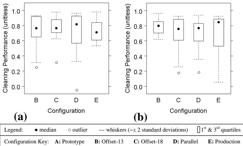
Figure 4. Cleaning performance versus configuration for the front orientation in corn residue. 'a' represents low speed (8 km/h) and 'b' represents high speed (10.4 km/h).
