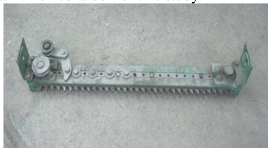
Figure 3- the actual view of the experimental cutter bar
