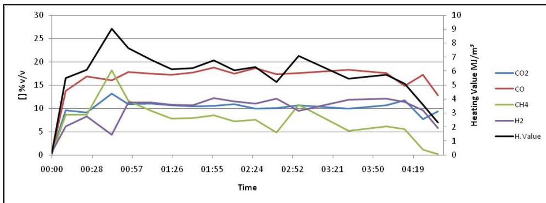
Figure 4 - Gas composition and calorific value as a function of time during the gasification test with Eucalyptus chips, Test3.
