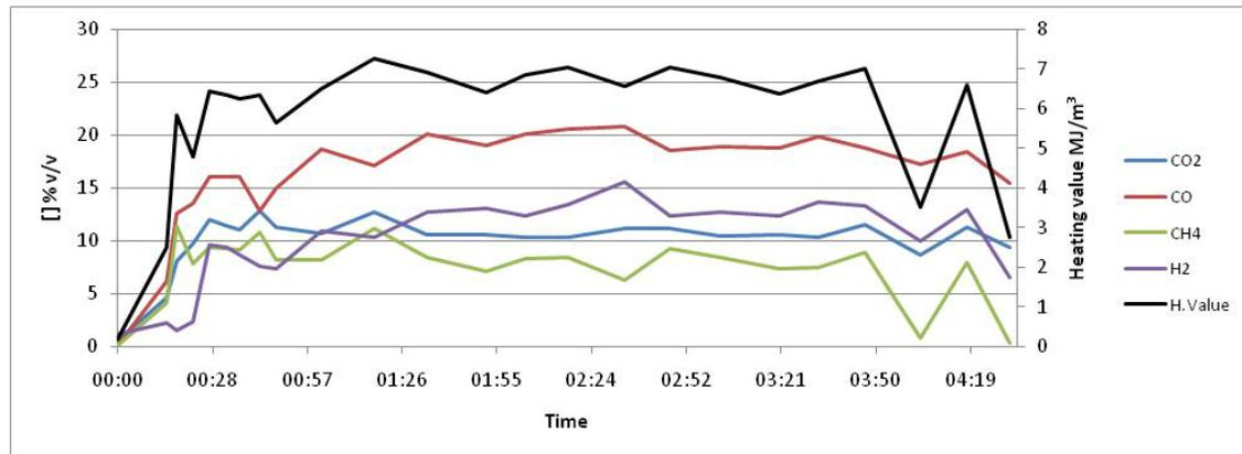
Figure 2 - Gas composition and calorific value as a function of time during the gasification of Eucalyptus chips, Test1.
