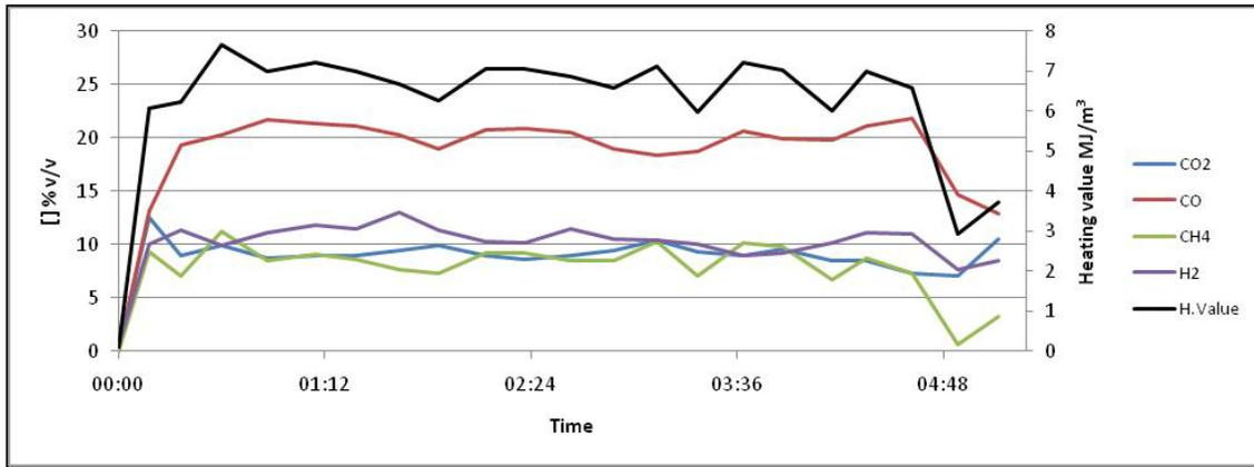
Figure 3 - Gas composition and calorific value as a function of time during the gasification test with Eucalyptus chips, Test2.
