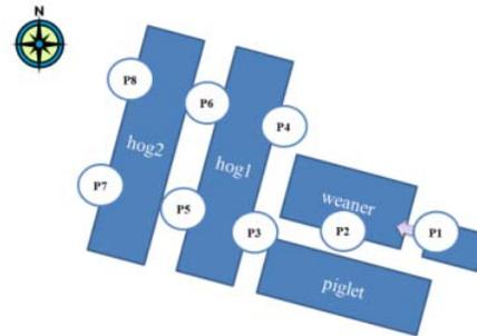
(b) Sampling points for virus test using air sampler with Teflon filters
