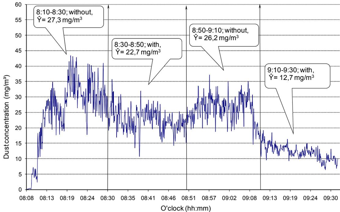
Figure 5. Run code D&C2. Dust concentration variation during filling of winter wheat in bulk loading bin without and with dust & chaff extractor.  $\hat{Y}$ = mean.
