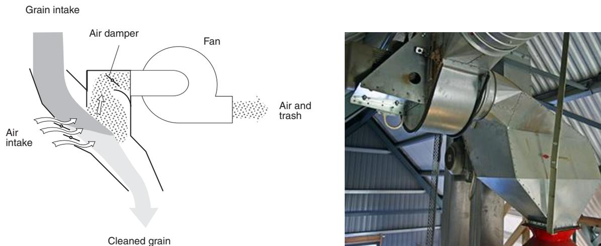
Figure 1. Dust & chaff extractor for dust reduction (Strand Mirza al. et. 1998; Qiuqing Geng, photo 2009).
