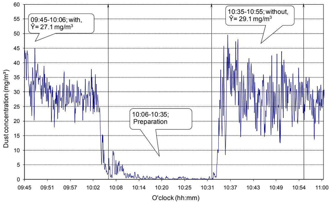
Figure 4. Run code D&C1. Dust concentration variation during filling of barley in bulk loading bin with and without dust & chaff extractor.  $\hat{Y}$  = mean.
