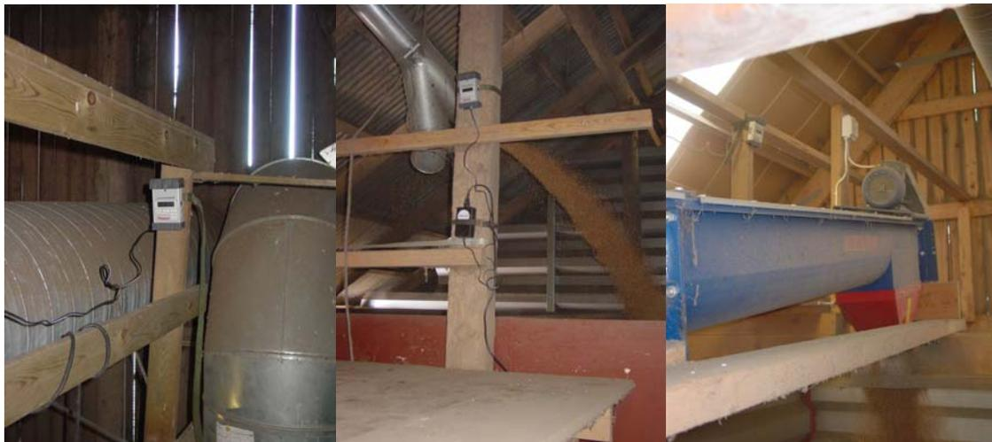
Figure 3. The measuring instrument, *personalDataRAM*, was installed approximate one meter from the conveyor outlet.
