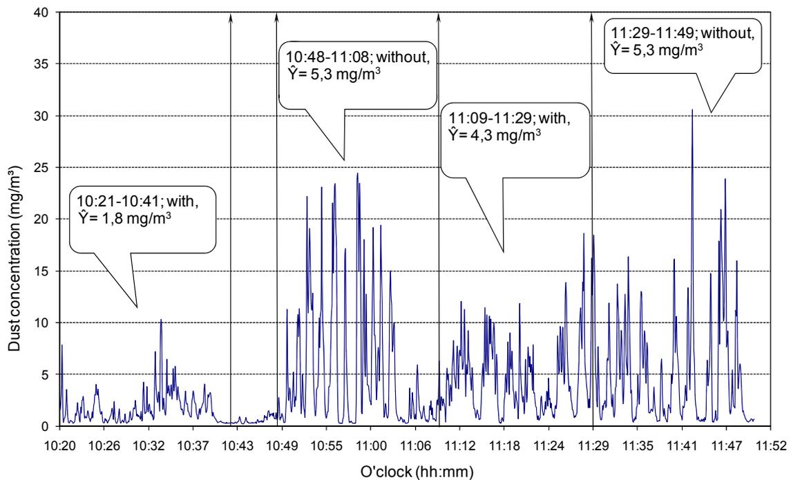
Figure 9. Run code ASP2. Dust concentration variation during circulation of spring wheat in grain dryer with and without aspirator.  $\hat{Y}$  = mean.
