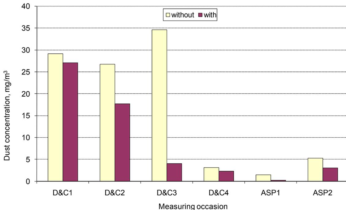
Figure10. Mean value for the dust concentration without and with equipment for dust reduction.
