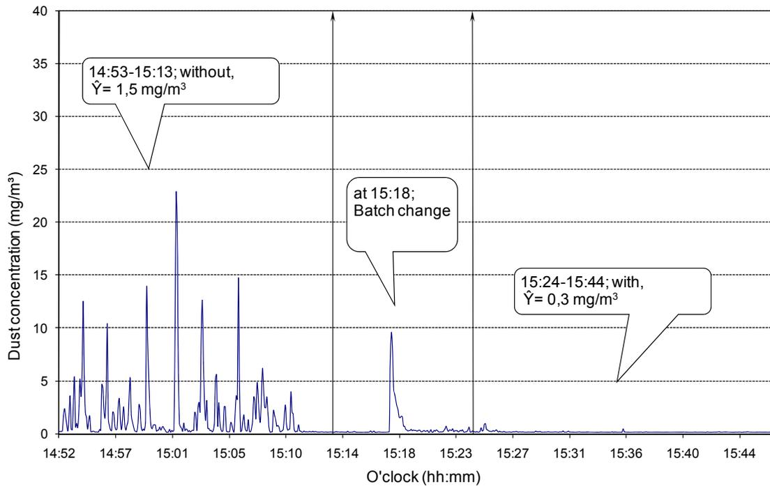
Figure 8. Run code ASP1. Dust concentration variation during filling and circulation of oat in grain dryer without and with aspirator.  $\hat{Y}$  = mean.
