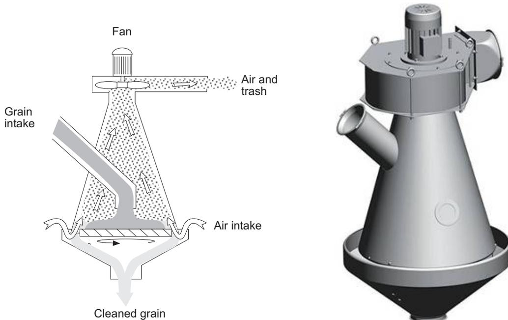
Figure 2. Aspirator for dust reduction (Strand Mirza al.et. 1998; [www.tornum.se](http://www.tornum.se)).
