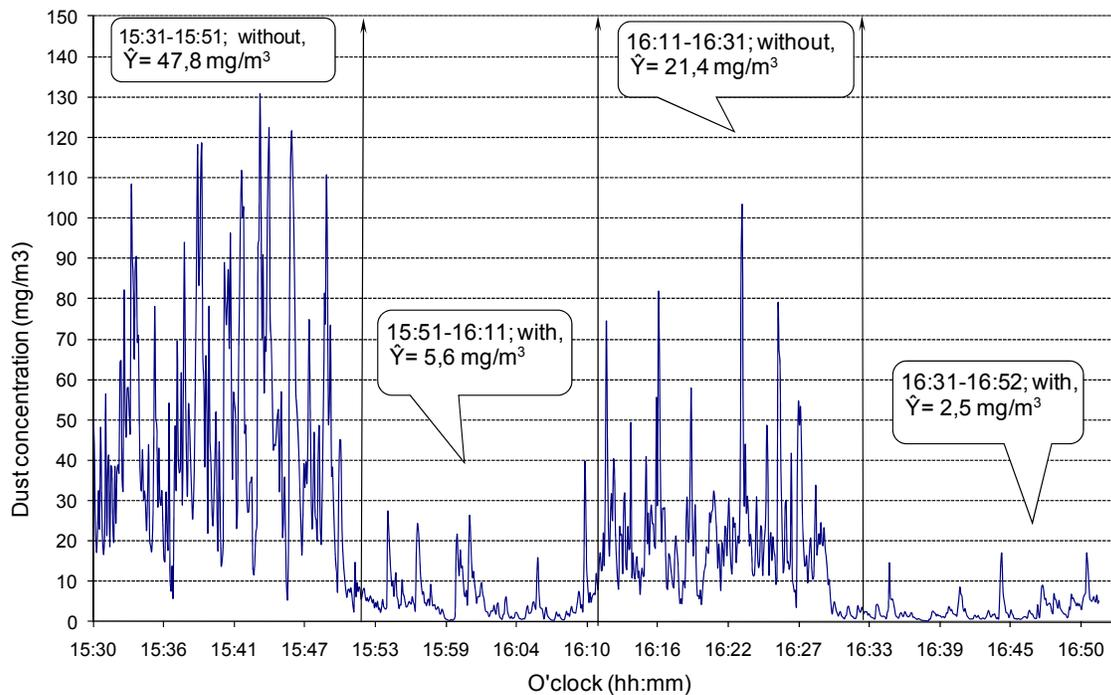
Figure 6. Run code D&C3. Dust concentration variation during circulation of barley in grain dryer without and with dust & chaff extractor.  $\hat{Y}$ = mean.
