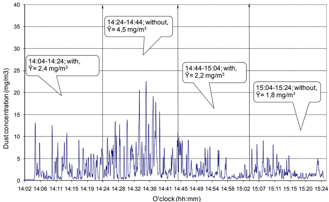
Figure 7. Run code D&C4. Dust concentration variation during filling of winter wheat in bulk loading bin with and without dust & chaff extractor.  $\hat{Y}$ = mean.
