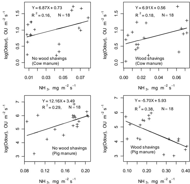
Figure 1. Relationship between odour and ammonia emissions from specific pig and cow manure compositions
