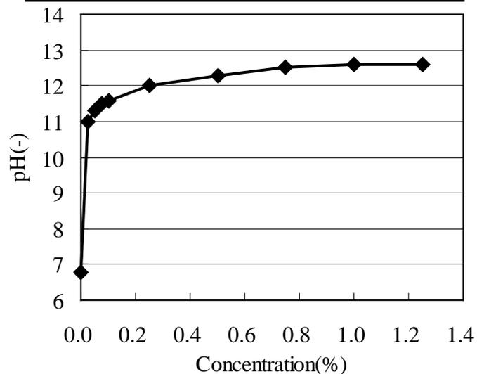
Figure 2. Value of pH in the solution and concentration of shell powder
