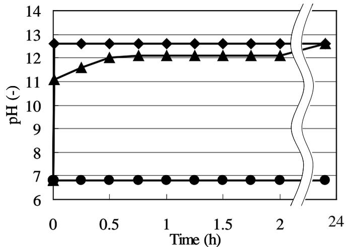
Figure 4. Value of pH in the solution which was put in shell powder (♦), film containing shell powder (▲) and blank film (●).
