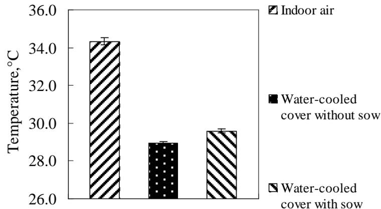
Figure 3. Black globe temperature of indoor air and the water-cooled cover with or without sow occupied during the hot period
