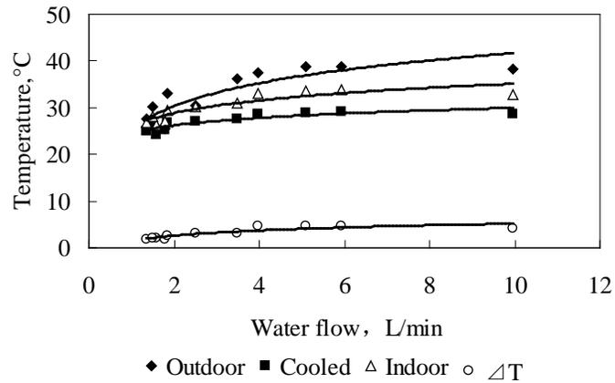
Figure 4. Relationship between the water flow and the outdoor temperature (Outdoor), indoor temperature (Indoor), water-cooled cover inside temperature (Cooled) and the temperature reduction of the sow occupied zone ( $\Delta T$ ).
