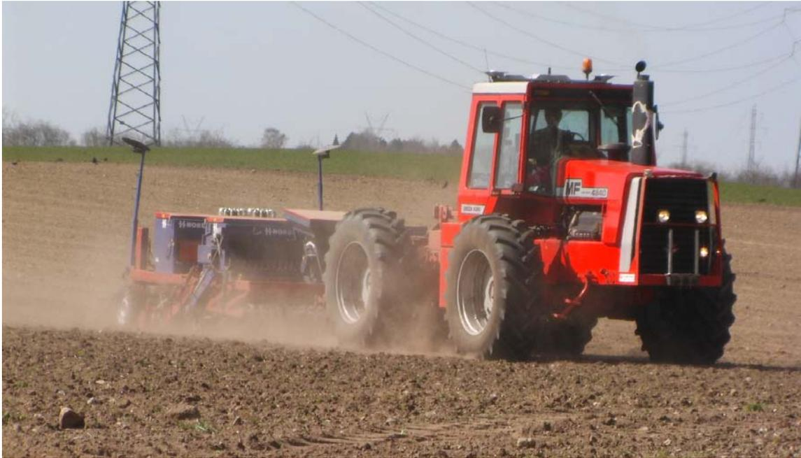
Figure 1. The tractor and seed used for establishment of the clover-grass crop in spring 2007. The tractor has been equipped with an RTK-GPS auto steering, making it possible to make a very precise establishment, with no traffic affecting within the plot.
