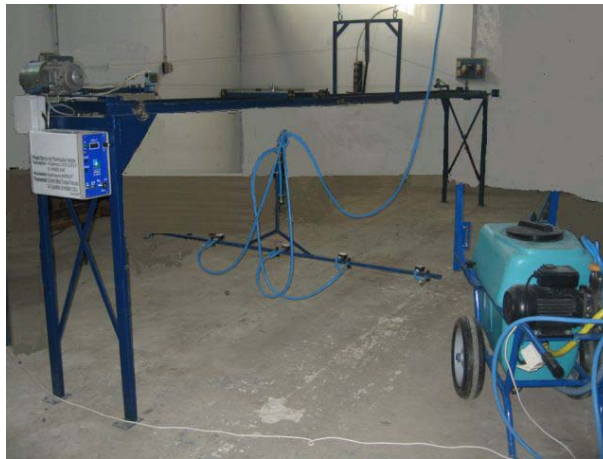
Figure 2. Mobile boom built to measure deposit under the weeds.
