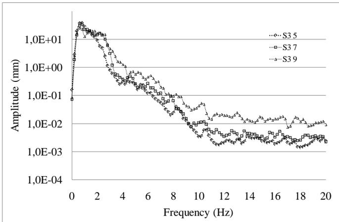
Figure 8. S3 surface frequency spectrum with respect to the forward speed.
