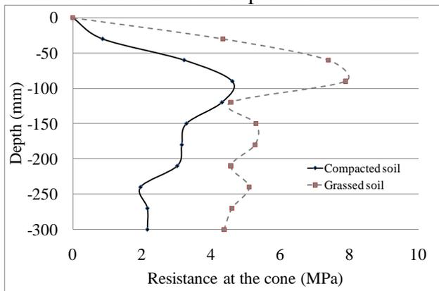
Figure 4. Resistance at the cone penetrometer of S1 and S2
