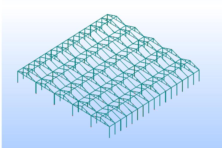
Figure 6. Proposed greenhouse structure
