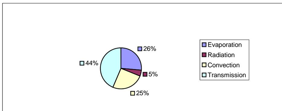
Figure 4. Sources of heat loss in breeding tanks
