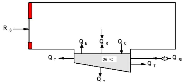
Figure 1. Heat Balance in breeding tanks
