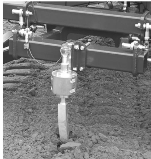
Figure 3. Sketch and photo of the cultivator tine with ultrasonic vibration.
