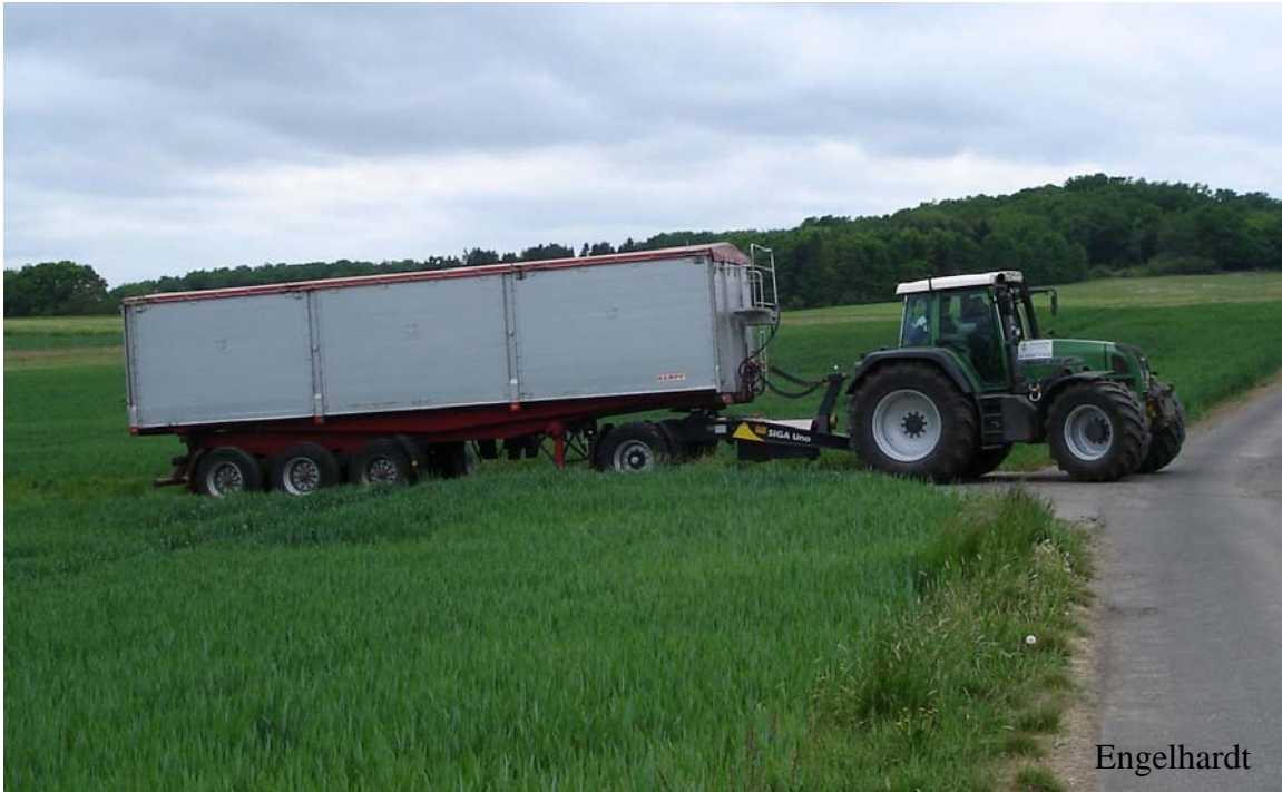
Figure 1: tractor and semi trailer with a connection trailer
