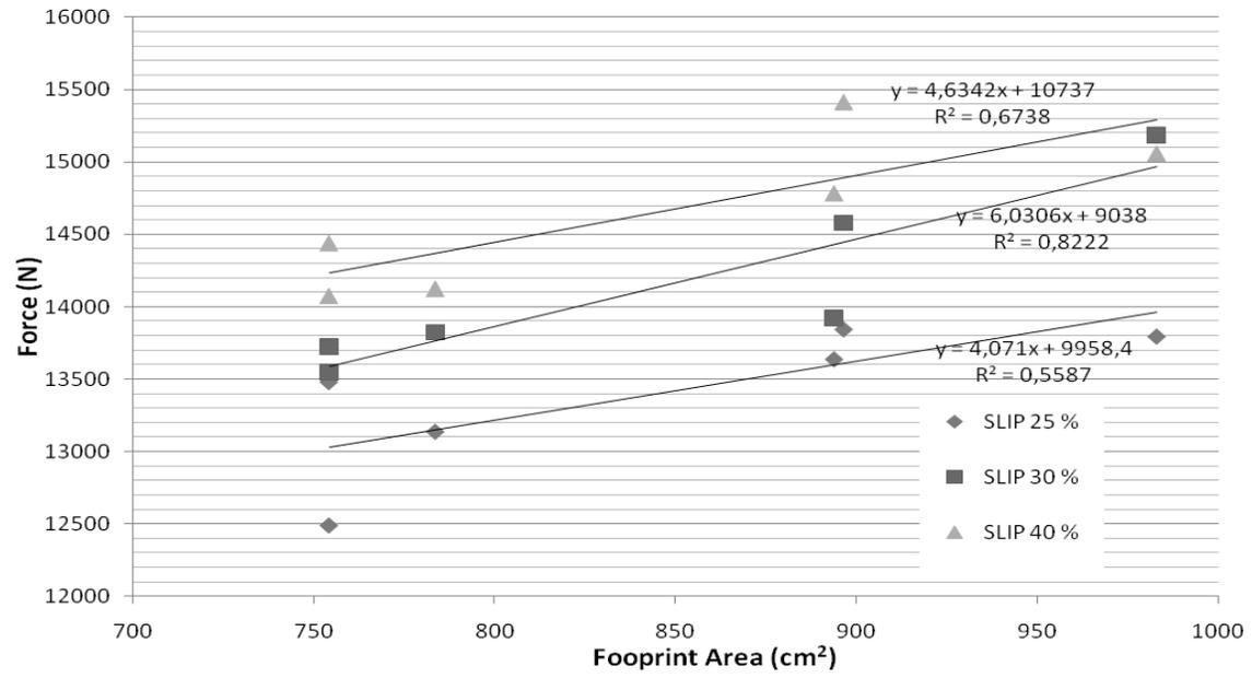
Figure 6: Dispersion between Single footprint (SF EL) and data from slippage test on grassy ground (S2).
