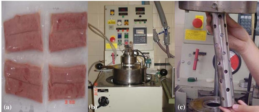
**Figure 1.** (a) Vacuum packaged turkey ham; (b) High pressure equipment; and (c) sample holder containing packaged turkey ham samples.
