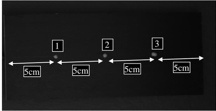
Figure 4: Knowing the exact dimension of the plate and the position of the particles on it enable to calculate the height of each particle.
