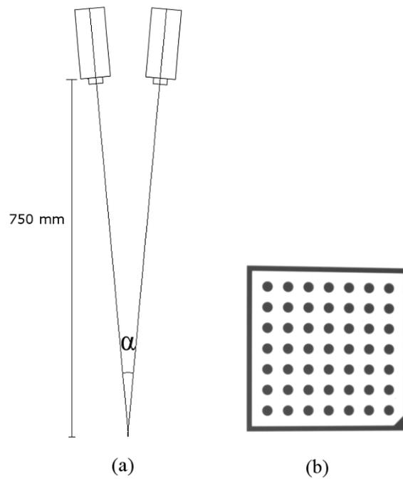
Figure 3: a) Stereo rig. b) 100x100mm<sup>2</sup> calibration plate.
