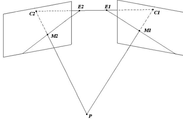
Figure 2: The epipolar geometry of a stereo rig.  $C1$ ,  $C2$ ,  $E1$ ,  $E2$ ,  $M1$  and  $M2$  are respectively the optical centers of the first and the second camera, the epipoles of the first and the second camera and the projection of point  $P$  on the first and the second image plane.  $E1M1$  and  $E2M2$  are respectively the epipolar lines of  $M2$  and  $M1$ .
