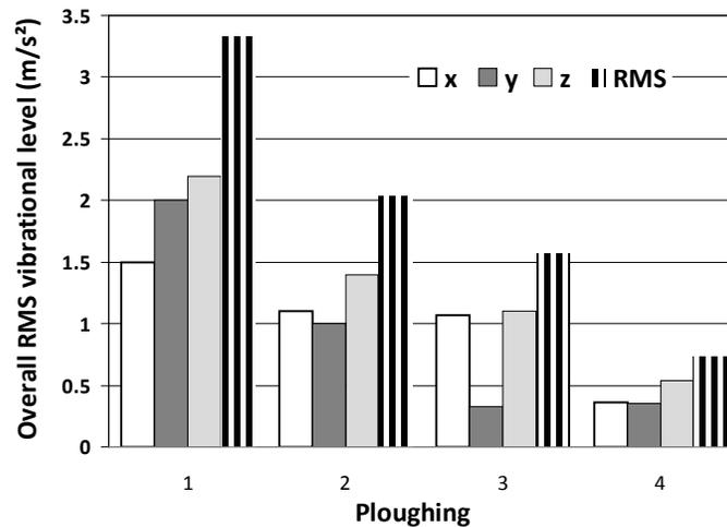
Figure 2. Whole-body vibrational levels measured on the tractor driver’s seat during ploughing.
