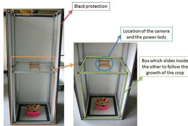
Figure 1. The new image acquisition system in our laboratory.
