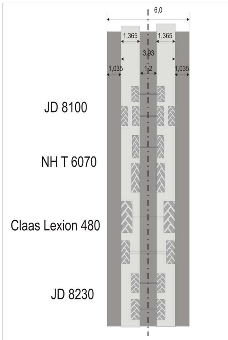
Figure A - 1 Track widths of used machinery (dimensions in meters)
